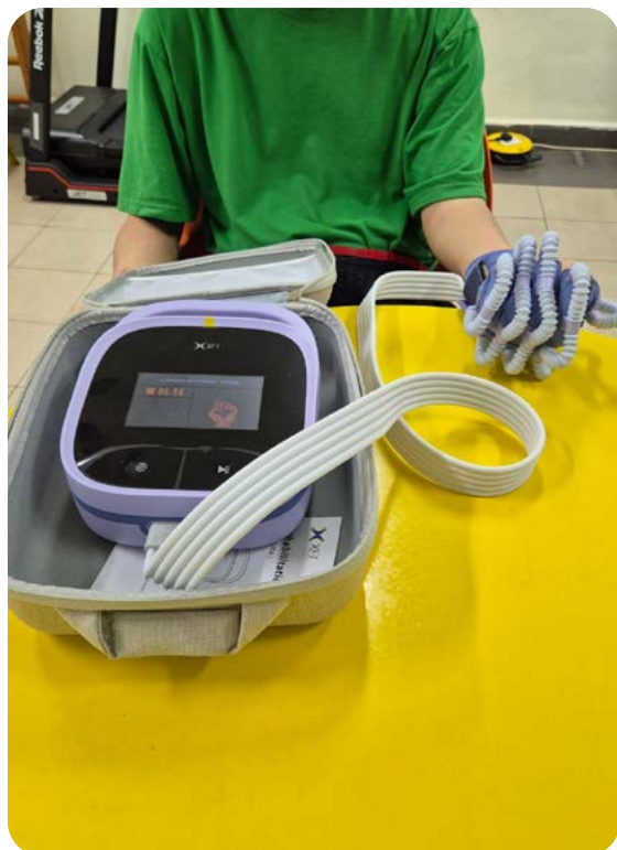
Robotic gloves used in hand rehabilitation for stroke patients
